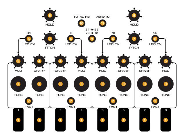
1 Sensors 1...8. Consist of a pair of contacts each. The upper contact is sensitive, the lower is the control voltage. Put your finger between the contacts to close the circuit with your body's conductivity. The current is very low, several orders below sensitivity threshold, and is absolutely safe:-)
