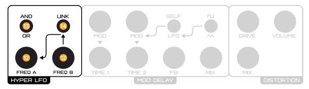
FREQ B. In upward position, FREQ A is multiplied by FREQ B, which is the logical operation AND. Both operations are conducted on a square waveform. The addition is analogue, and the LFO output signal has a gradient.
